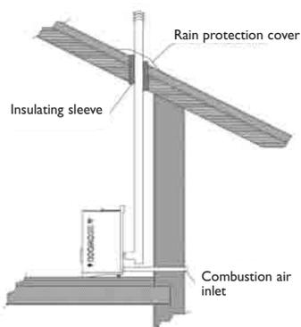
If the stove is to be installed in an existing chimney flue built into the wall, the pipe should be installed along the whole length of the chimney flue in order to prevent condensation that would mark the walls.
