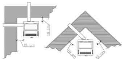
If the stove is positioned near a wood-lined wall or the gas exhaust pipe is in contact with similar material, insulate the material with suitable fireproof or fire-resistant products.
