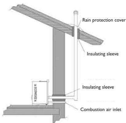
If the gas exhaust pipe is installed as in the drawing on the right, a rain protection cover will be needed in addition to the requirements listed above.
