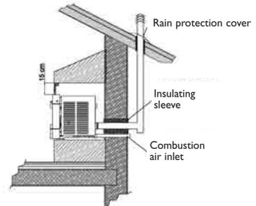
If the stove is installed in a building with potentially inflammable walls, it will be necessary to place an insulating sleeve between the wall and the flue gas exhaust pipe and similarly for the overhanging part of the building's roof.
