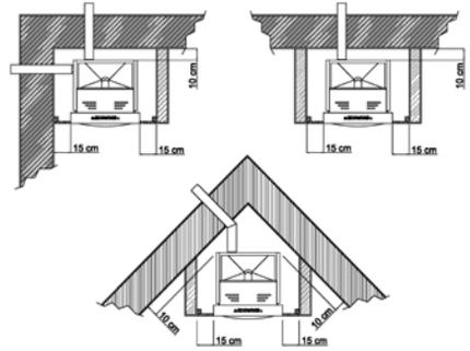
Connect the flue pipe of your stove to an existing chimney or, alternatively, install a fume exhaust pipe outside the building. The pipe must have a minimum pipe diameter of 80 mm and reach higher than the top of the roof.
